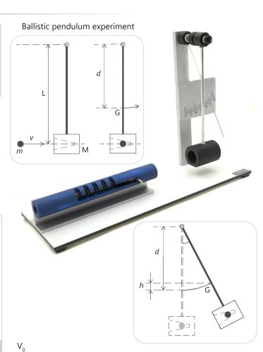
The launching system is removable and suitable to verify the initial speed of a projectile according to the laws of parabolic motion; this allows to compare the result with that one obtained by performing the inelastic collision experience.
