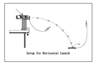
2. Adjust the angle of the Projectile Launcher to zero degrees so the ball will launch horizontally.
