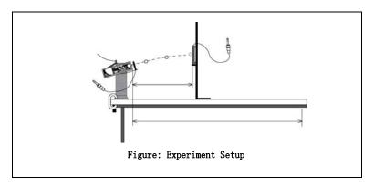
2. Adjust the angle of the Projectile Launcher to any desired angle.
