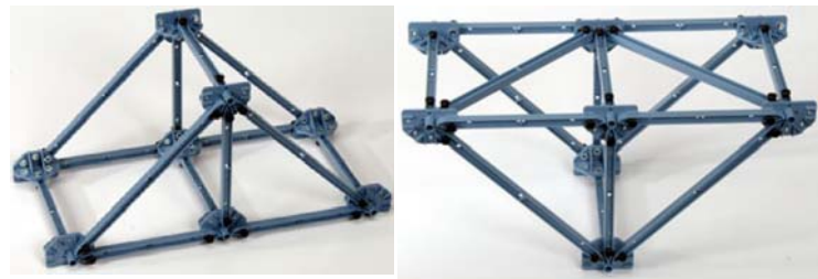
Figure 14: (Left) A three-dimensional kingpost truss structure. (Right) Kingpost truss with cross bracing.
