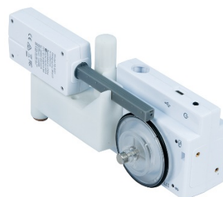
Figure 3: Magnetic Field Sensor Mounted on the Rotary Motion Sensor
