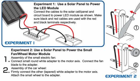
**3.** Connect the solar panel to the circuit board then to the motor base as shown. The fan may need to be flicked with your finger to start.
